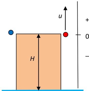
For the red ball: it reaches the ground at time  $t$  given by  $-H = ut - \frac{1}{2}gt^2$ .
